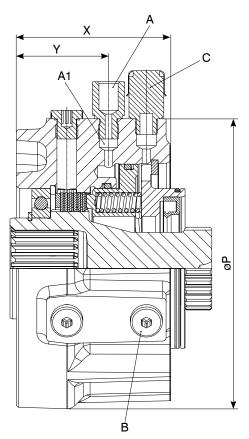
A = with adapterA1 = without adapter Our gear units can be supplied with hydraulically released negative multidisc brakes.
